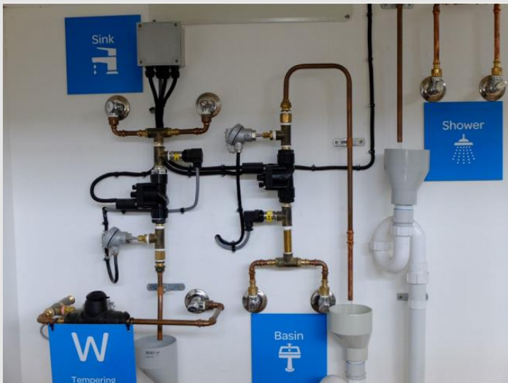
Figure: Trialling of rainwater to hot water connections at Holmesglen TAFE
