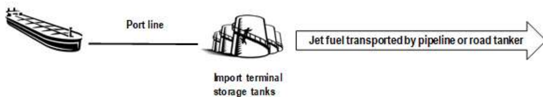
FIGURE 2.3 GENERAL ARRANGEMENT FOR AN IMPORT TERMINAL
