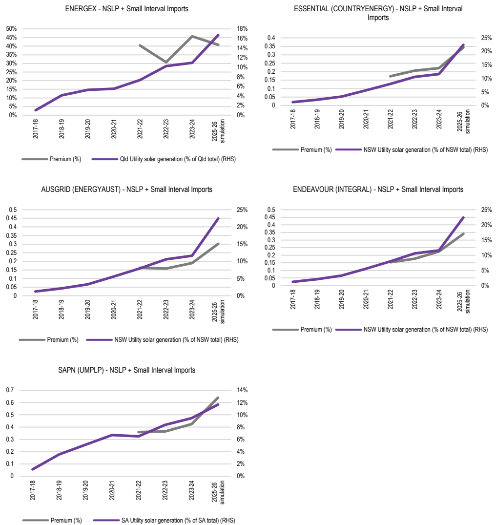
Figure 4.19 Simulated annual DWP for NSLP and Interval meter demand as a percentage premium of annual TWP for 2025-26 compared with range of actual outcomes in past years, and market share of utility scale solar (%)
